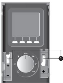
Wall mounting Secure the thermostat using the screws and pegs or fit onto a flush-mounted box (1, distance between centres 60 mm).
